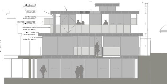
HOUSE A, Northern Elevation (Rear) (Scale 1:100)
